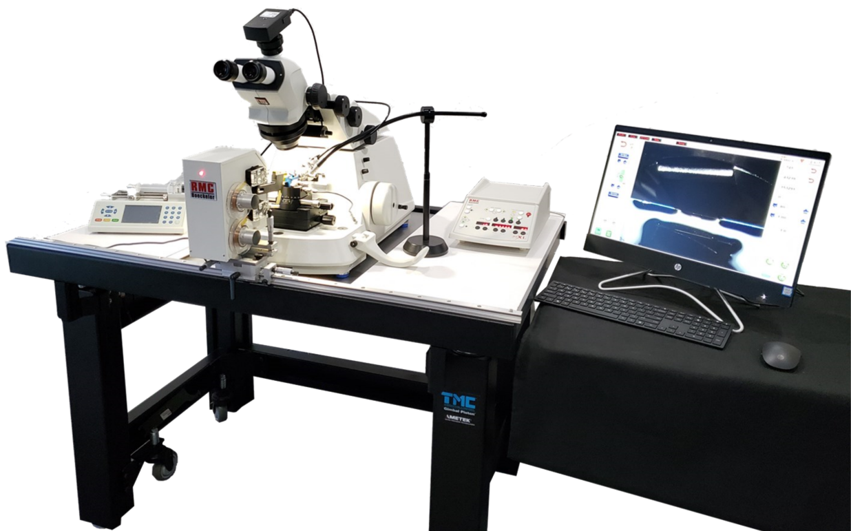
Figure 2. The RMC Boeckeler ATUM unit in operation with the PT PCZ ultramicrotome.
